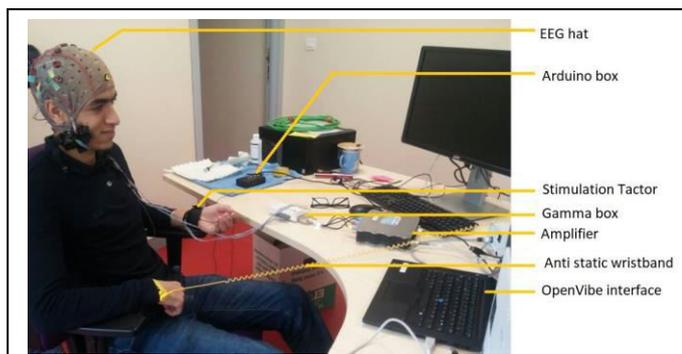
Figure 2: Hardware and software for our experience setup.
