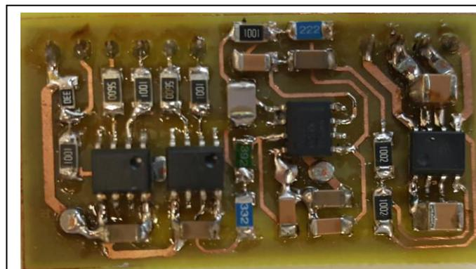
Figure 7: Sine wave generator electronics board (left), 2x C-2 Tactor connected to the Arduino box including the wave generators (right).
