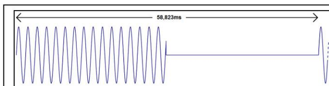
Figure 5: One period of a 17Hz burst of 274,12Hz sine wave output with a pulse ratio of 50%.
